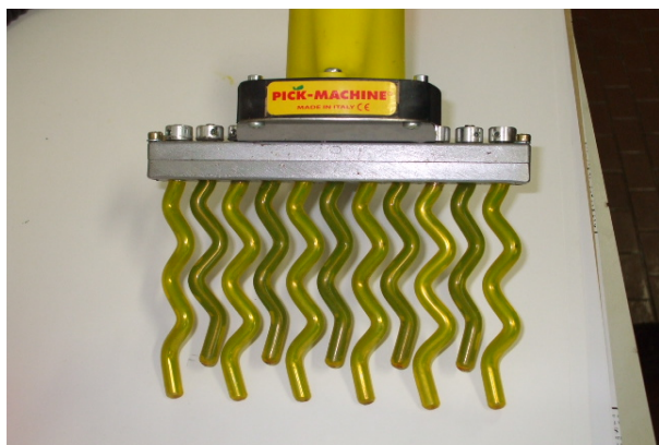
Figure 2 Equipment utilized for the harvest of myrtle berries produced by COIMA-(Italy)
