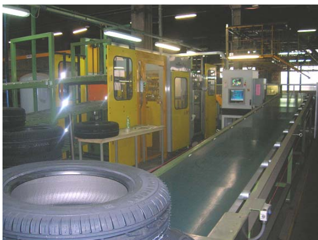
Figure 24 The Model AIT Tyre Dynamic Balance System (courtesy of Marangoni Tyre S.p.A).
